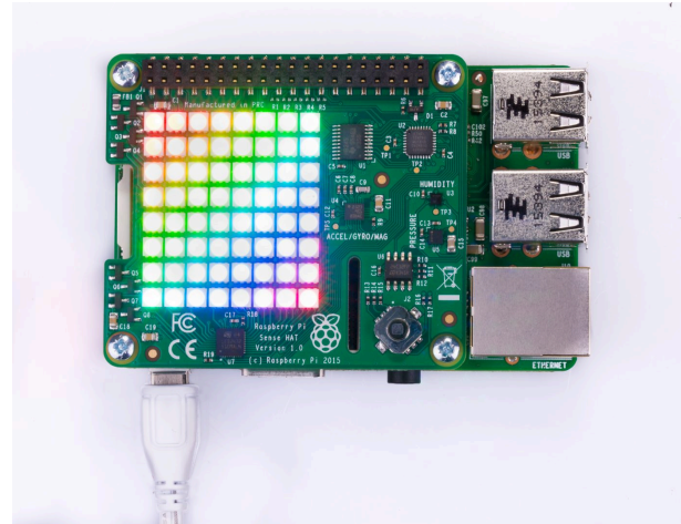
Figure 2: Photo of a Raspberry Pi with a Sense HAT attached on it[9].
